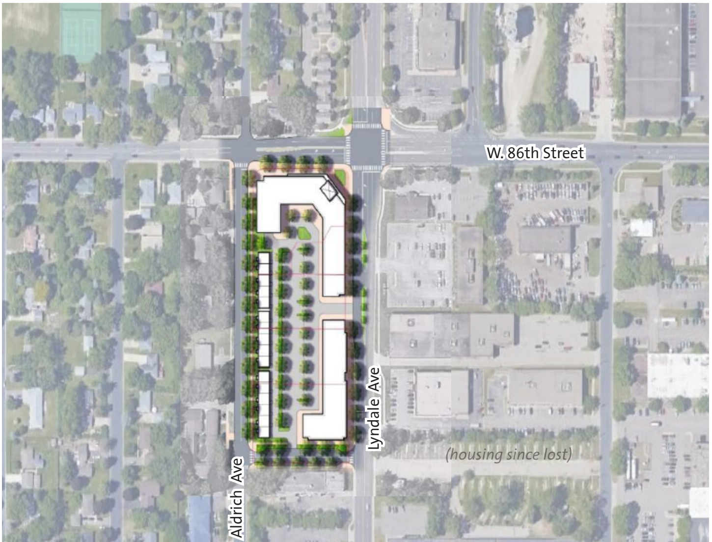
86th Street Redevelopment Concept. Townhomes provide a transitional buffer between existing single family homes and higher density residential and mixed use fronting Lyndale.
