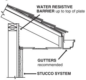
4. All laundry, bathroom, furnace and fireplace vents, pipes, lights, hose bibs, etc. that extend through the walls or are placed on the exterior wall must be in place and flashed **prior** to the installation of the water resistive barrier. The general contractor must coordinate the sub-contractors so these items are not installed after the fact, leaving openings for potential moisture intrusion. See Figure 3 below.
