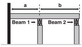
Solution: Use "a" or "b", whichever is greater, to determine joist size. Use "a" + "b" to determine the size of Beam 1 and the post footing size for the posts supporting Beam 1.
