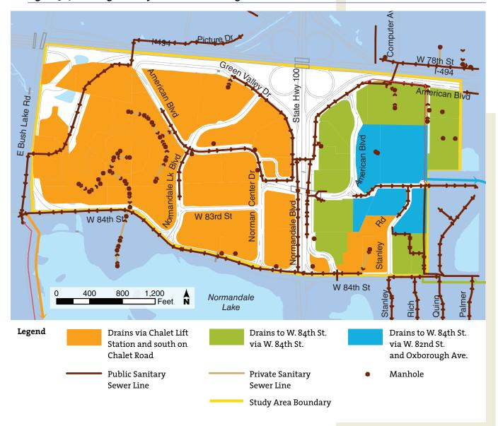
Figure 3.4 Existing Sanitary Sewer and Drainage Areas
