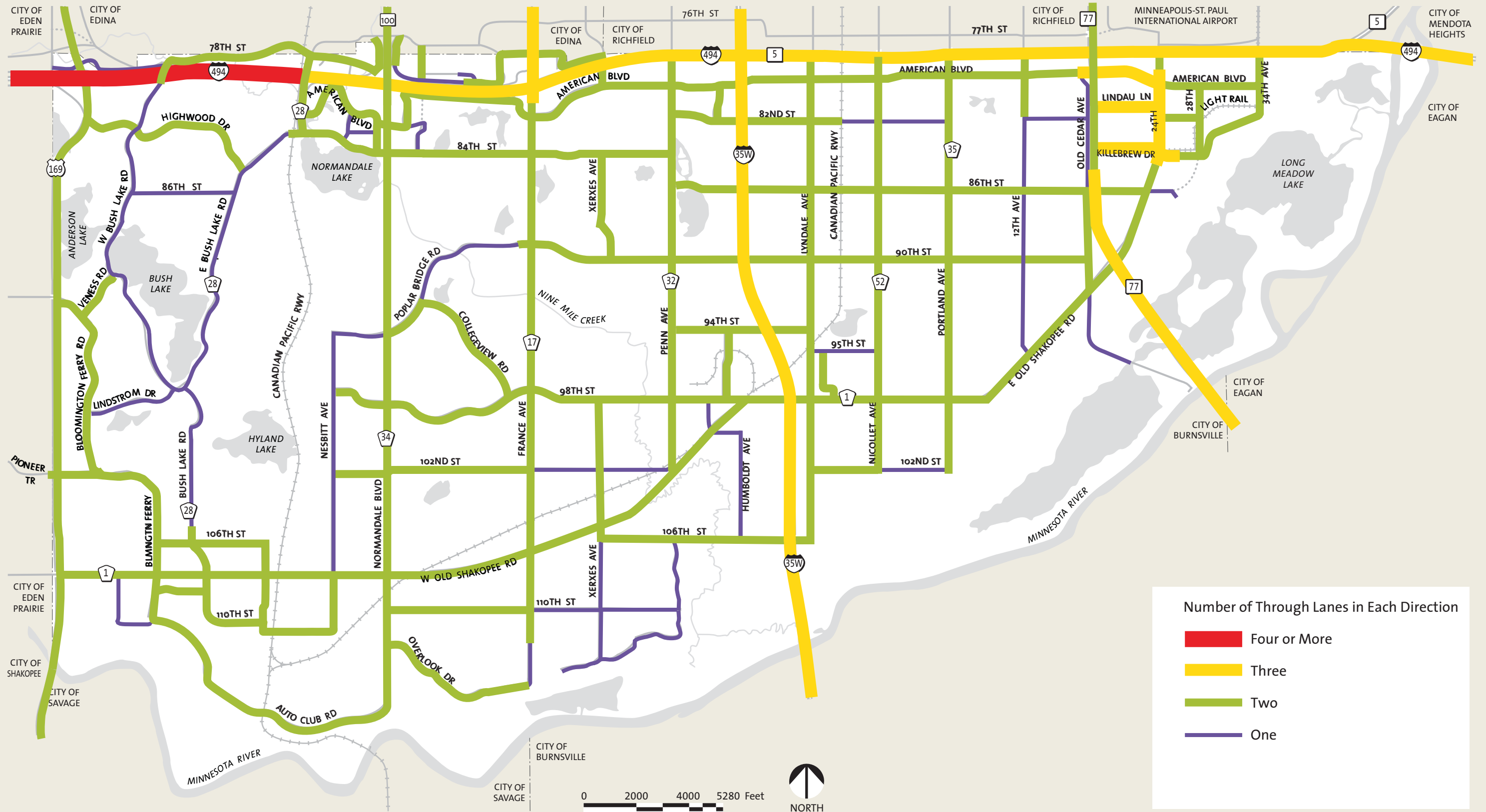
Figure 4.9 Existing Through Lanes in Each Direction
